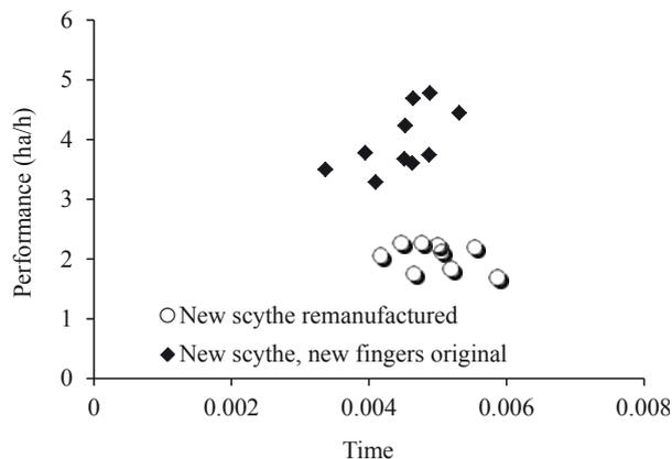
Fig. 1. Dependence of performance on cutting mechanism condition
