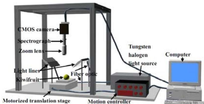
Figure 2. Sketch of the hyperspectral imaging system
