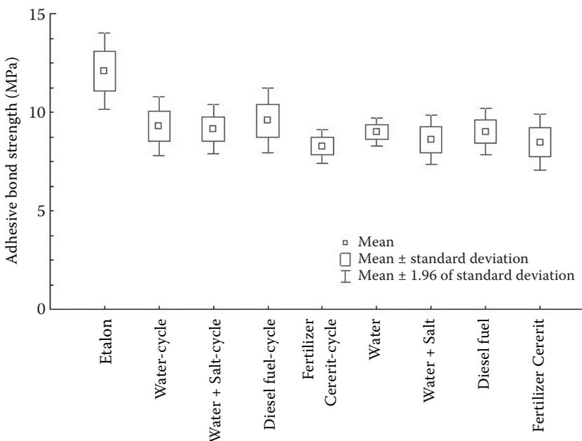
Fig. 9. Influence of degradation medium on the bonded joint strength
