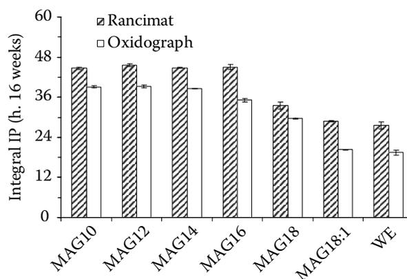
Figure 2. Oxidative stability of FBs with MAGs determined by Rancimat (A) and Oxidograph instrument (B) during storage time
