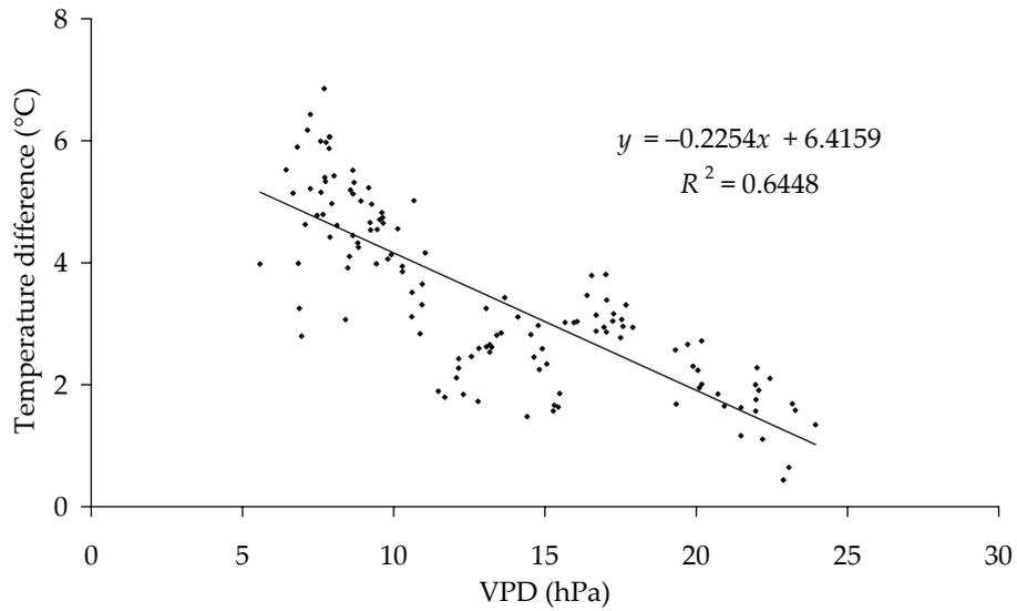
Figure 7. Correlation of temperature difference (°C) with vapour pressure deficit (hPa) in a rainless period around midday (11:00–14:00), at global radiation intensity > 700 W/m<sup>2</sup>, Klečaty, 6.5.–16.6.2005
