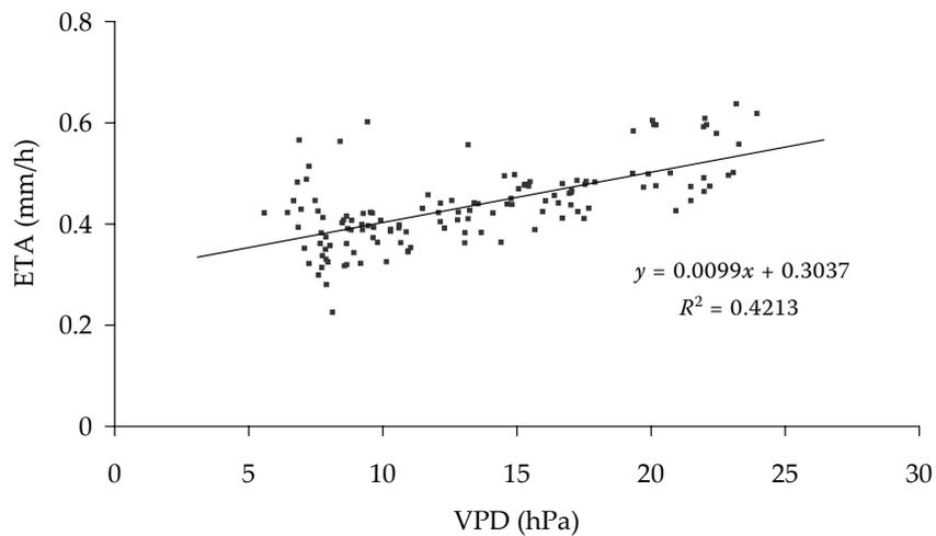
Figure 8. Correlation of actual evapotranspiration rate with vapour pressure deficit in a rainless period around midday (11:00–14:00), at global radiation intensity > 700 W/m<sup>2</sup>, Klečaty, 6.5.–16.6.2005
