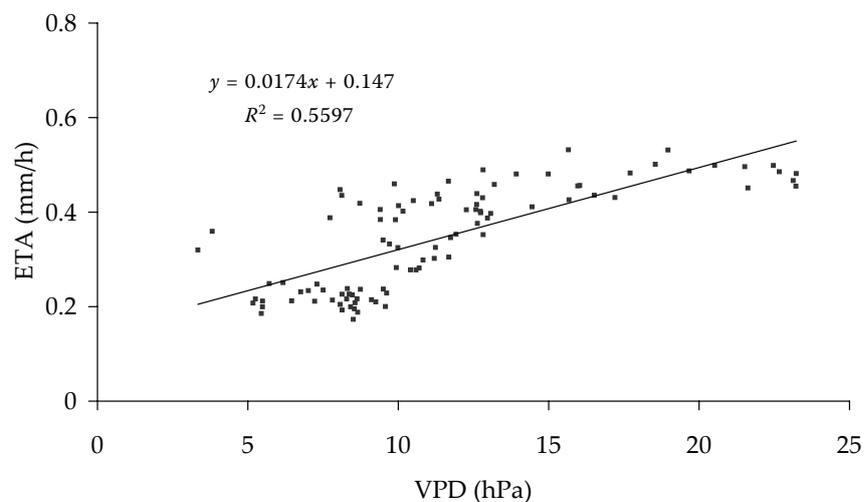
Figure 3. Correlation of actual evapotranspiration rate with vapour pressure deficit in a rainless period around midday (11:00–14:00), at global radiation intensity > 700 W/m<sup>2</sup>, Klečaty, 1.4.–6.5.2005
