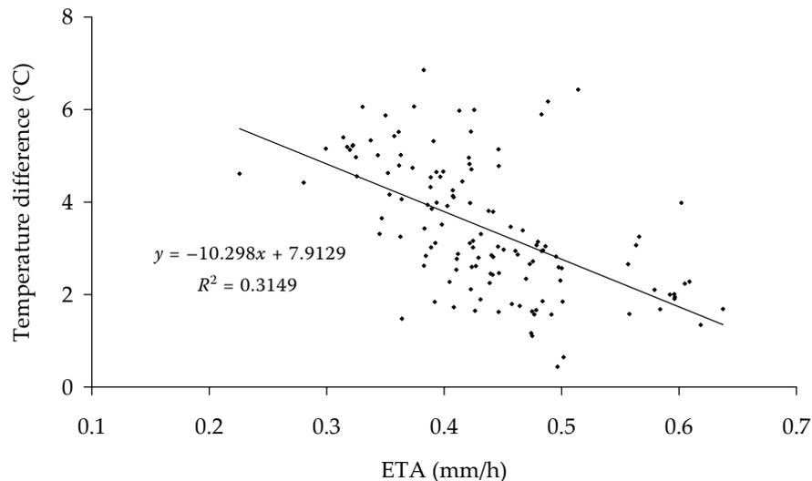
Figure 9. Correlation of temperature difference (°C) with actual evapotranspiration rate (mm/h) in a rainless period around midday (11:00–14:00), at global radiation intensity > 700 W/m<sup>2</sup>, Klečaty, 6.5.–16.6.2005
