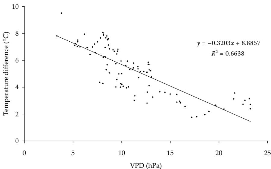
Figure 2. Correlation of temperature difference (°C) with vapour pressure deficit (hPa) in a rainless period around midday (11:00–14:00), at global radiation intensity  $> 700 \text{ W/m}^2$ , Klečaty, 1.4.–6.5.2005
