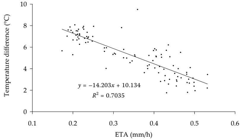
Figure 4. Correlation of temperature difference (°C) with actual evapotranspiration rate (mm/h) in a rainless period around midday (11:00–14:00), at global radiation intensity  $> 700 \text{ W/m}^2$ , Klečaty, 1.4.–6.5.2005
