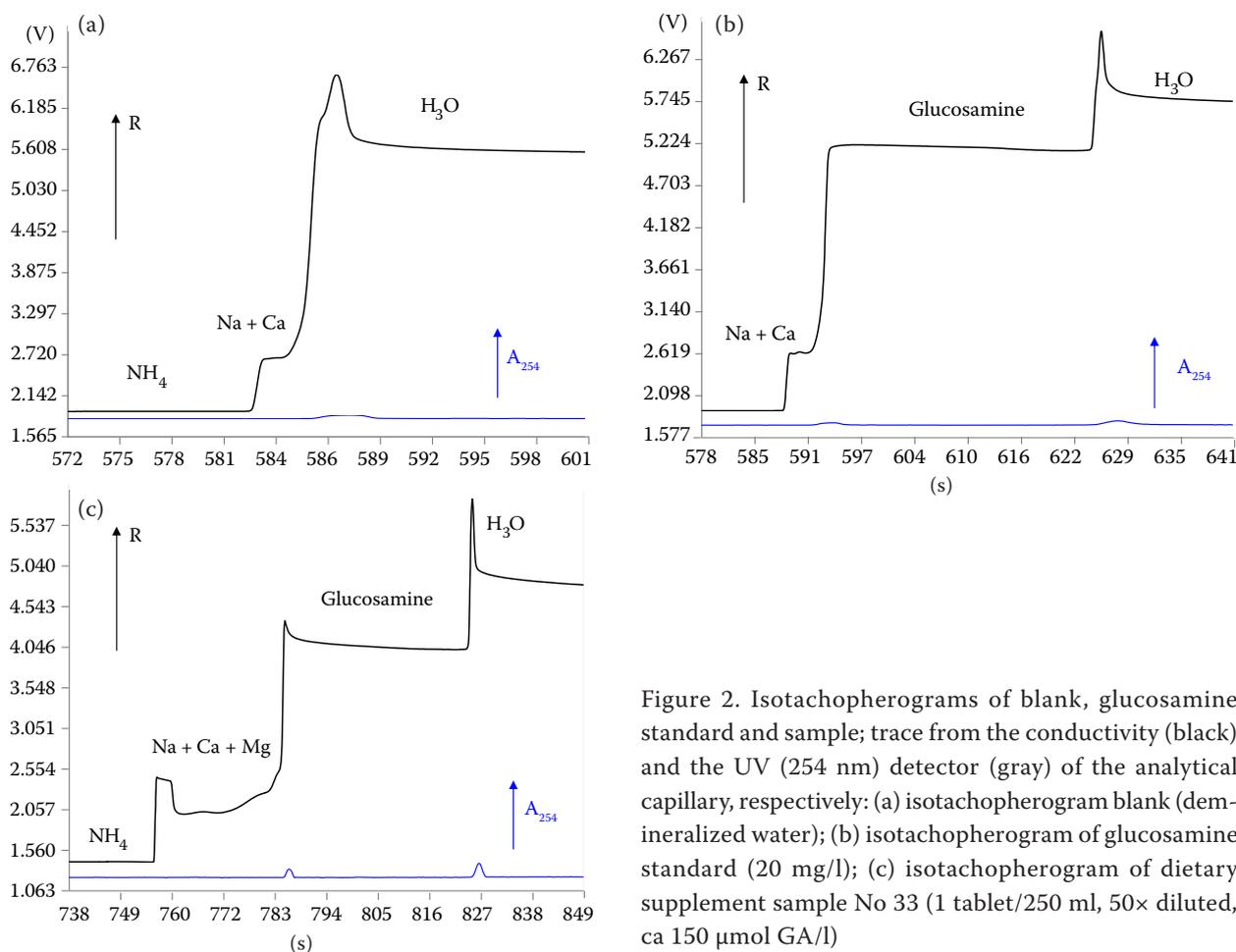
Figure 2. Isotachopherograms of blank, glucosamine standard and sample; trace from the conductivity (black) and the UV (254 nm) detector (gray) of the analytical capillary, respectively: (a) isotachopherogram blank (deminerallized water); (b) isotachopherogram of glucosamine standard (20 mg/l); (c) isotachopherogram of dietary supplement sample No 33 (1 tablet/250 ml, 50× diluted, ca 150  $\mu$ mol GA/l)
