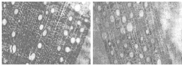
Fig. 4. Variation in the disposition of the pores of *Quercus ilex* Linnaeus in internal (a) and external (b) area
