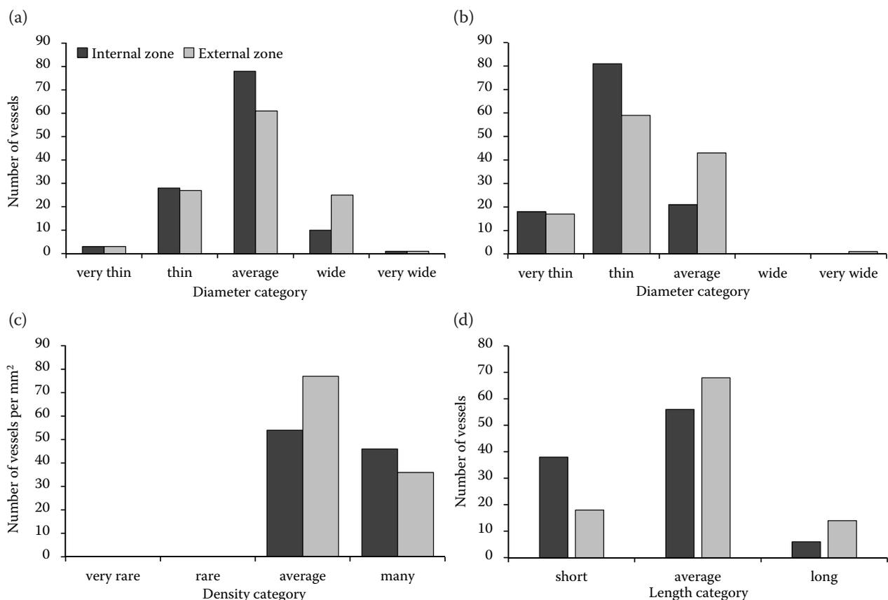
Fig. 5. Histograms of wood characteristics of the vessels: diameter in early wood (a), diameter in latewood (b), density (c), length (d)
