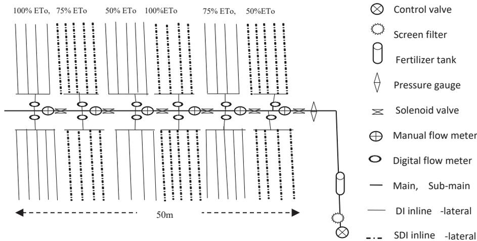
Figure 1. Irrigation system with units of the surface and subsurface drip irrigation with inline drip laterals under the deficit irrigation regimes
