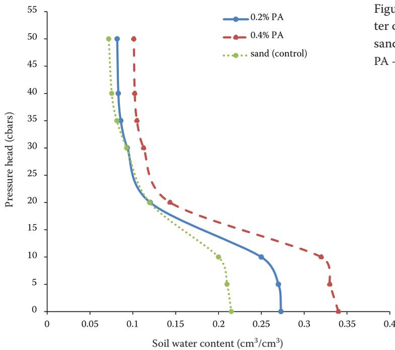
Figure 3. Polymer addition effects on the soil water content and pressure head of the site medium sandy soil
