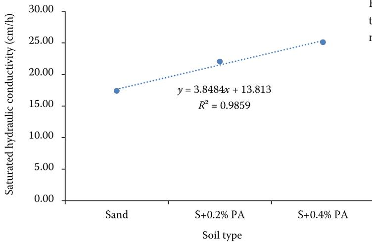
Figure 4. Impact of the polymer additions on the saturated hydraulic conductivity of the site’s medium sandy soil
